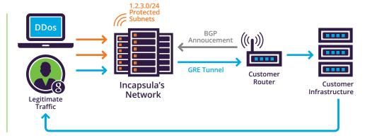
Traffic flowing via Incapsula during a DDOS attack. BGP announcement is used to route protected subnets through Incapsula for mitigation.
